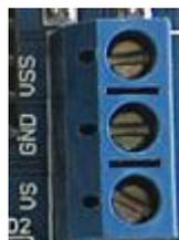
The servo can be powered through the VS input power in the figure above, and the input voltage should be adjusted with the need of the motor, for the input is to power the servo directly. For example, if you use the TR213 servo, the input voltage should be adjusted to 4.8V-7.2V, the voltage over this range would burn your servo. In order to avoid unnecessary losses, please operate in strict accordance with the instructions!
